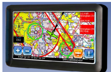
Figure 7 Typical Moving-Map GPS Display. Credit: Airbox
