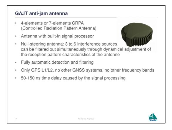
The GAJT (pronounced: gadget) anti-jam antenna will automatically detect and filter out 3 to 6 simultaneous interference sources, depending on the exact GAJT model. The GAJT is designed for only the GPS L1+L2 bands, so even if the connected receiver is capable of handling other systems/frequency bands, it will only get the GPS L1+L2 signals from the GAJT antenna.
