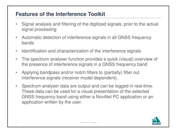
The automatic spectrum analysis function is running continuously on any OEM7 receiver to monitor the environment, even when the specific spectrum analysis logs are not being requested by the user. When an interference signal is detected, the receiver will toggle a status flag. For now, the receiver will not automatically apply filtering to mitigate an interference source.
