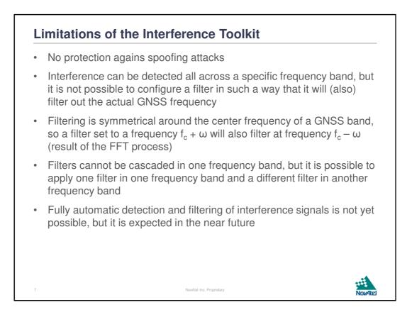
The spectrum analysis data are covering all of the GNSS bands "allowed" by the receiver model. When a filter is applied, the frequencies of the actual GNSS signals are protected by not allowing the filter settings to filter out any of the actual GNSS frequencies. If this protection had not been implemented, it would have been possible to (accidentally) filter out the signals needed for the actual positioning.
