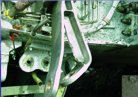
Pylon Rear Mount Bulkhead Fitting
